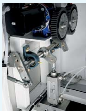
Traino film con brushless Film pulling device with brushless
